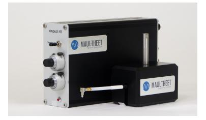
With the new **vImpact-61**, structures can be excited precisely and reproducibly. The excitation forces are measured with the load cell in the hammer head, which is suitable for frequency ranges up to 60 kHz. This makes the small modal hammer particularly interesting for acoustic and laser measurements.
